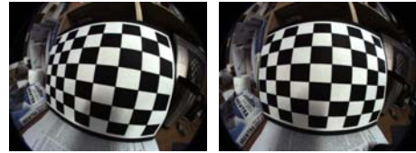
Fig. 4 Several samples for finding distorted coefficients After calculations using Open CV, correction matrix, K is found to be
